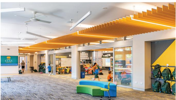
To make the classroom spaces flexible and simple to adapt, Alspec ProGlide Ultra Flat Sliding Doors were installed for both internal and external interfaces. Functioning as both access doors and 'openable walls', the doors were configured with four large panels (one fixed and three sliding). The wide-spanning doors allow a classroom to expand into a larger open space when needed or easily closed to create a more delineated environment, while natural light is maintained at all times.
